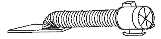
Air should be blown into a space that contains a hazardous atmosphere. Remember that contaminants are likely heavier or lighter than air. Blowing air into a space will agitate and help evaporate the contaminants and disperse them throughout the space. A space under positive pressure will eventually expel the contaminant through any openings in the space. Theoretically, air blows a distance of 30 diameter times farther than it can be exhausted.
